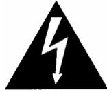
**WARNING: HIGH VOLTAGE!!** This control must be installed in a GROUNDED enclosure. Provide a safety interlock on door to remove power before gaining access to device. The ground/earth connection can be made to the 110-Z3 chassis mounting point on heat sink / side panel.
